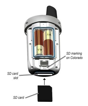
Inserting an SD Card into the Colorado
