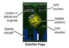
The blue bars on the Satellite page indicate that the Colorado has "locked" on a satellite. White bars indicate that the Colorado is still collecting ephemeris data.
