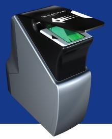
MorphoWave<sup>™</sup> Desktop is a contactless fingerprint acquisition solution. This innovative device captures four finger images with a single movement in less than a second. Its dynamic acquisition capability allows subjects to be 'on the move' during fingerprint capture. MorphoWave<sup>™</sup> Desktop is well suited for high traffic environments.
